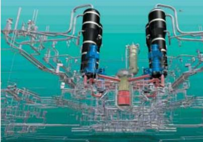
**The European Pressurized Water Reactor (EPR)** is a further development of the conventional pressurized water reactor type. It is designed for the generation of 1600 MW and an operating life of 60 years. The illustration above shows 3D data generated by PDMS of Aveva.
